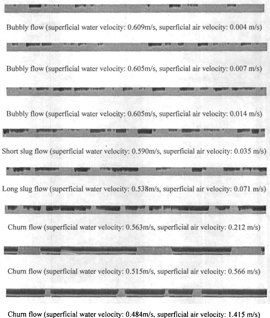
Fig. 3 Flow patterns vs. different air flowrates (black denotes air phase and grey denotes water phase)
