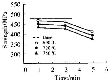
Fig. 2 Strength of aluminized specimen vs hot dip time and temperature
