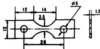
Fig. 1 Tensile specimen for SEM in-situ observation
