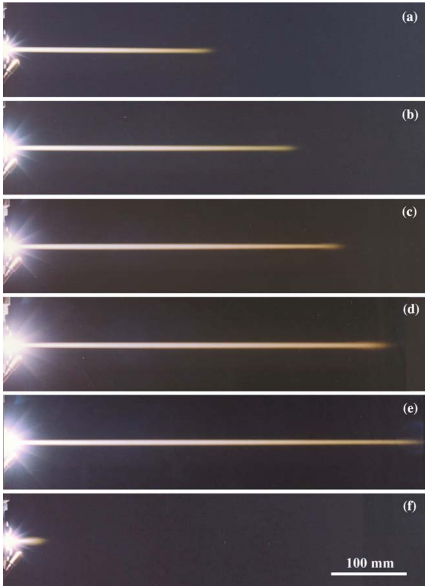
Fig. 1 Variation of the visual plasma jet length with the argon flow rate. (a)–(f) correspond to the argon mass flow rates of 1.7, 2.1, 2.4, 2.7, 2.9 and 3.7 \times 10^{-4} kg/s. Arc current 200 A
