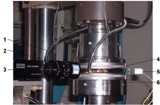
Fig. 1. The experimental set-up for observing rock damage and rupture, 1—illumination, 2—camera, 3—CCD, 4—AE sensors and rock sample, 5—extensometer, 6—platens of MTS810.
