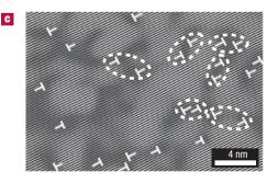
micrographs showing dislocations in a nanostructured aluminium grain (120 nm in diameter) produced by a large deformation. a, Contrast due to the presence of strain caused mainly by dislocations. b, High-magnification view, with dislocations marked (T). Note the circled dislocation dipoles. c, Fourier-filtered image of another grain. The ellipses show examples of dislocation dipoles.
