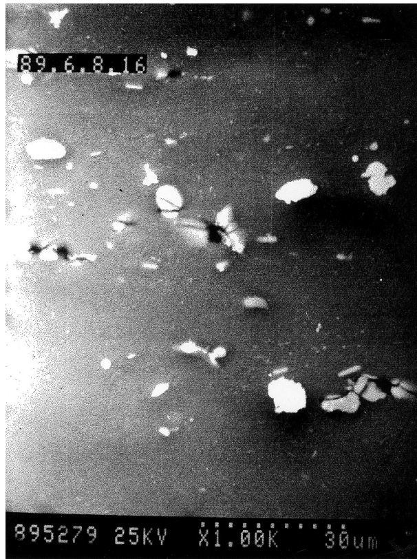
Fig. 1. Microcracks on the section of an impacted aluminium alloy specimen (impact velocity: 593 m/s, tensile stress: 7460 MPa, time duration: 142.2 ns).
