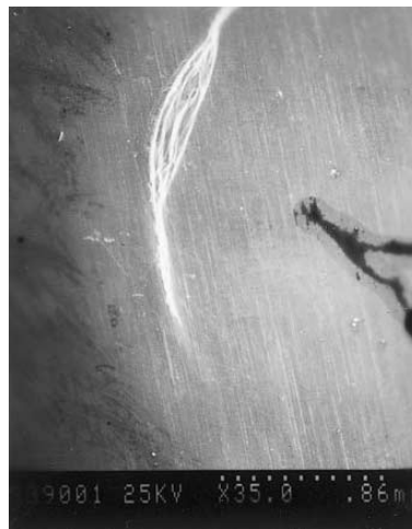
Fig. 7. Photograph of brass foil failure by plugging viewed from the rear surface with a laser energy of 29 J over a region 4.5 mm in diameter.
