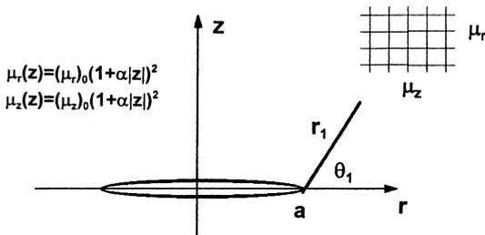
Fig. 1. Penny-shaped crack in transversely isotropic FGM.
