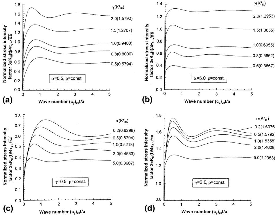
Fig. 3. Normalized stress intensity factor versus wave number for (a) α = 0.5, (b) α = 5.0, (c) γ = 0.5 and (d) γ = 2.0.
