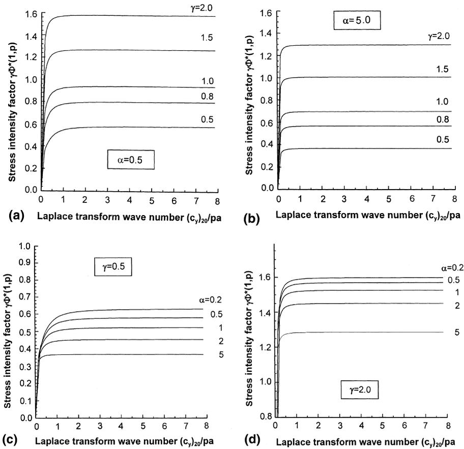
Fig. 2. Variations of stress intensity factor in Laplace transform plane for (a)  $\alpha = 0.5$ , (b)  $\alpha = 5.0$ , (c)  $\gamma = 0.5$  and (d)  $\gamma = 2.0$ .
