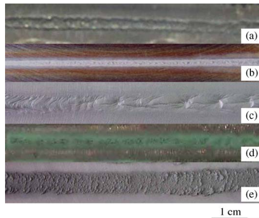
Fig. 1. Appearance of the remelting tracks on the stainless steel surface (a); cast iron surface (b) and Al–Si alloy surface (c). Appearance of the cladding tracks on the stainless steel surface (d) and Al–Si alloy surface (e).
