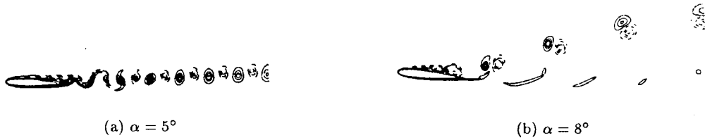
图 3 M_\infty = 0.5, Re = 10^4, t = 28 时 NACA0012 翼型绕流涡量等值线 Fig.3 Contours of vorticity for a flow past NACA0012 at M_\infty = 0.5, Re = 10^4, t = 28
