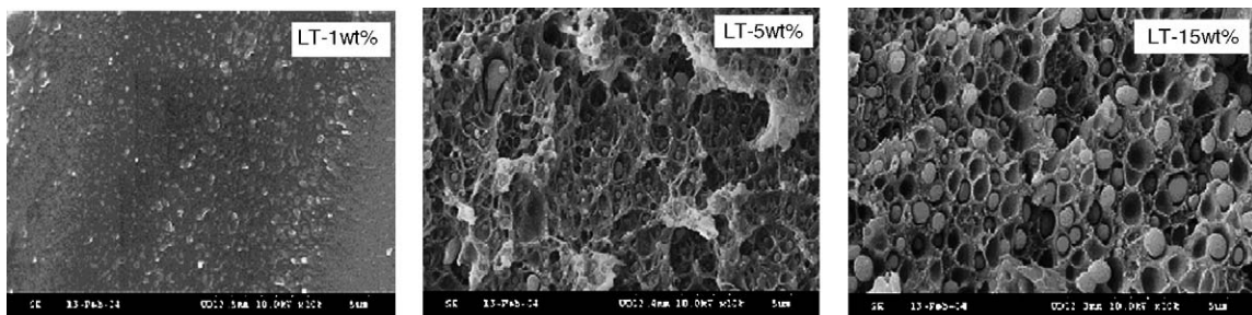
Fig. 6. Fractured surface morphology of composite films with different silica contents at 77 K.
