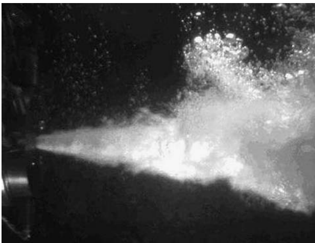
Fig. 4 Image of instantaneous flow pattern of high-speed air jet in still water
