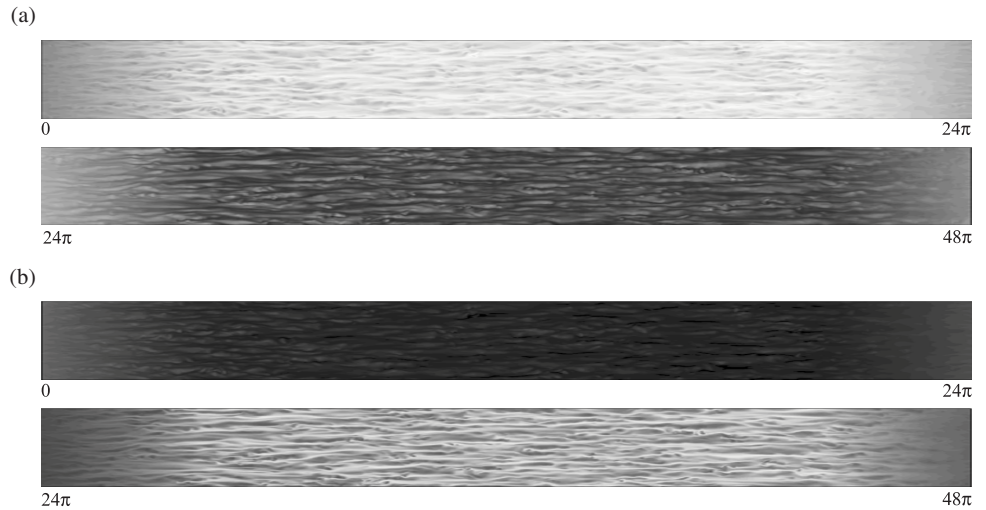
Fig. 12 Distribution of kinematic viscosity (a) and thermal conductivity (b) at y^+ \approx 5 for case1.
