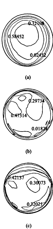
Fig.8 Cross-section oil volumetric fraction in the branch
