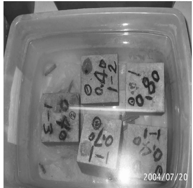
Fig. 1. Specimens are immersed in sulphate solution.
