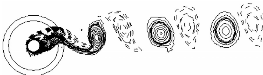
Fig. 17. Instantaneous vorticity contours of the flow over a rotating circular cylinder at q = 1.57 ; solid and dashed lines denote positive and negative contours, respectively.
