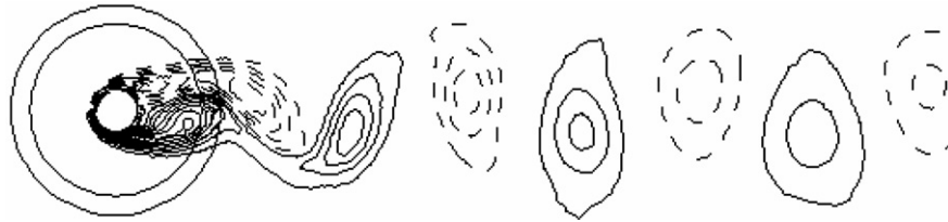
Fig. 10. Instantaneous vorticity contours of the flow over a fixed cylinder at Re = 100 ; solid and dashed lines denote positive and negative contours, respectively.
