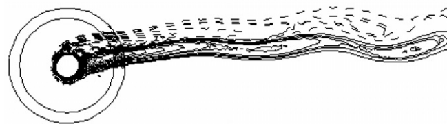
Fig. 20. Vorticity contours of the flow over a rotating circular cylinder at q = 2.0 ; solid and dashed lines denote positive and negative contours, respectively.
