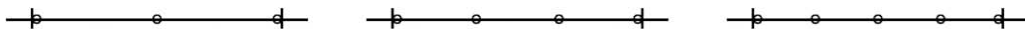
Fig. 1. The locations of the unknowns in one dimension for the third-order (left), the fourth-order (middle) and the fifth-order (right) schemes.
