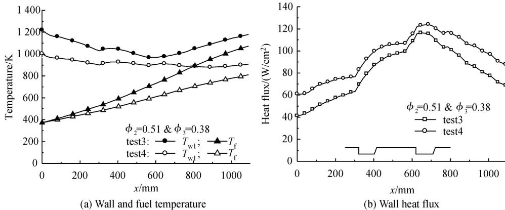
Fig 5 Results of test3 and test4 with dual injections
