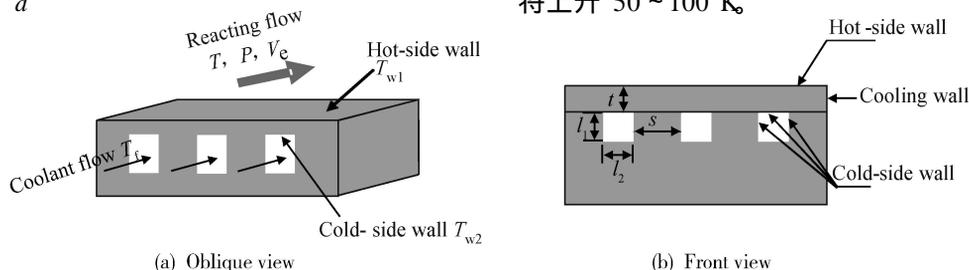
Fig 2 Schematic diagram of the cooling configuration
