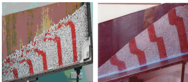
图 5 堆积体试验破坏形态 Fig.5 Failure forms of accumulation body test
