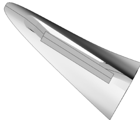
Figure 3 Optimized waverider configuration.
