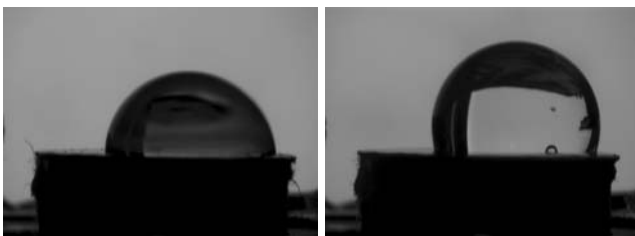
Fig. 8 Water drops on PTFE: drop created during 1g on left picture, drop created during microgravity on the right picture
