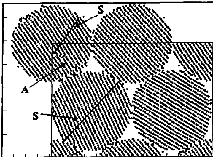
Figure 10. Relaxed atomic structure after consolidation of nanocrystalline \alpha -iron (9.4 nm, 17923 atoms, 4 preset dislocations).
