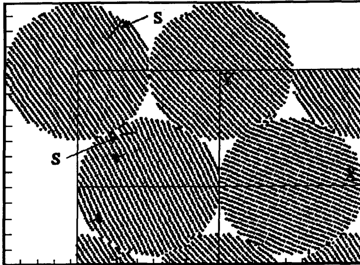
Figure 9. Relaxed atomic structure after consolidation of nanocrystalline \alpha -iron (12.78 nm, 29756 atoms, 3.6 GPa, without preset dislocations).
