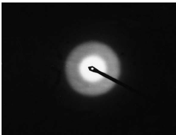
Fig. 3. Electron diffraction pattern of the a -alloy coating (0.25 mm deep from the top surface).
