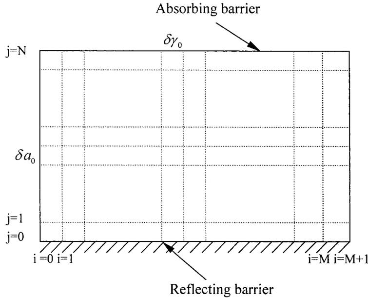
Figure 2. Rectangular mesh for finite difference scheme.
