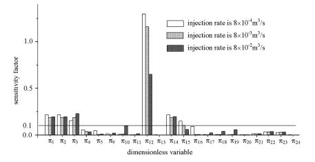
dimensionless variables with injection rate. The results are plotted in Fig. 3, showing that  $\pi_1, \pi_2, \pi_3, \pi_{12}, \pi_{14}, \pi_{15}, \pi_{16}$  are the dominant variables for low injection rates, and  $\pi_1, \pi_2, \pi_3, \pi_{12}, \pi_{14}, \pi_{15}$  and  $\pi_1, \pi_2, \pi_3, \pi_{10}, \pi_{12}, \pi_{14}$  for moderate and high injection rates, respectively.
