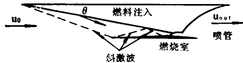
图 2 三波内压式超燃发动机示意图 Fig.2 Schematic of the integrated SCRAMJET with a three-shock diffuser
