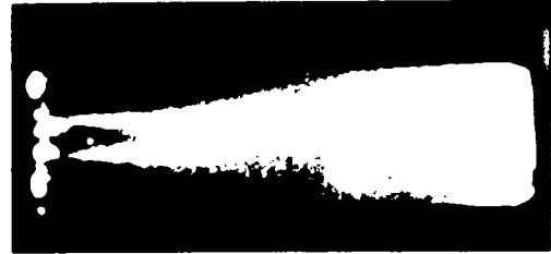
Fig. 5 Picture of 2D supersonic diffusion flame with parallel H 2 injection
