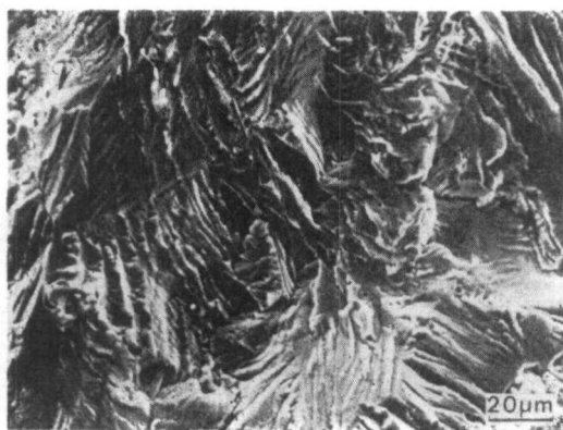
图 6 近门槛值的低速扩展的断口形貌，周期解理和塑性撕裂 Fig. 6 Slow propagation rate fracture topographic feature, cyclic cleavage and plasticity tear
