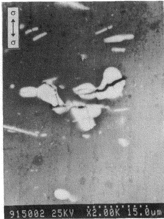
Fig. 5. The nucleation develops from the fringe of the particles into their interior ( \sigma = 7470 MPa, \Delta T = 112 ns).
