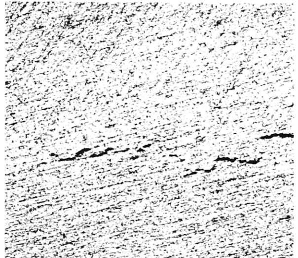
FIG 4. Crack feature of specimen with F = 1/2 magnification \times 50 .
