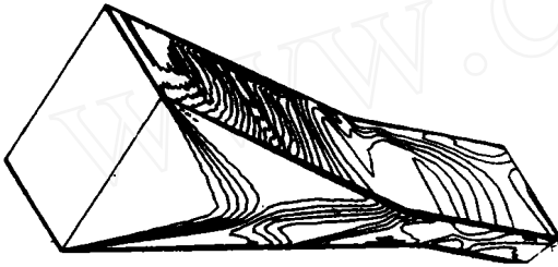
Fig. 4 3D Mach contour ( Ma = 5 )
