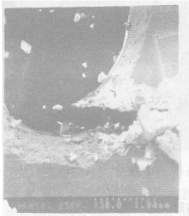
图 7 大理岩破坏后孔边断裂 SEM 像 Fig. 7 Fracture SEM photo of hole boundary in marble after failure
