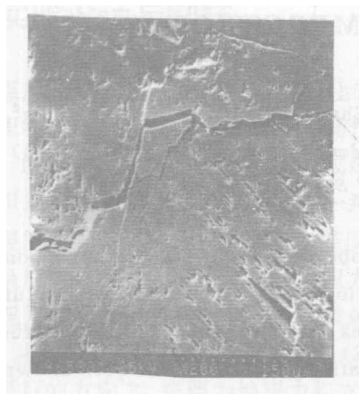
图 14 裂纹折曲处块状破裂 SEM 像 Fig. 14 Micro-fracture SEM photo of fold with lump failure
