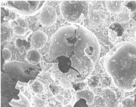
图 5(a) 横截面内的孔边裂纹 Fig 5(a) Cracks at the edge of a cell hole (in transverse section)
