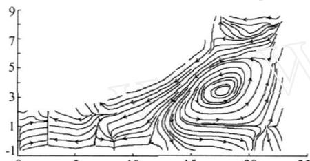
(b) 热端附近流线  $h_0 = 4.6\text{mm}$ ,  $\Delta T = 20^\circ\text{C}$
