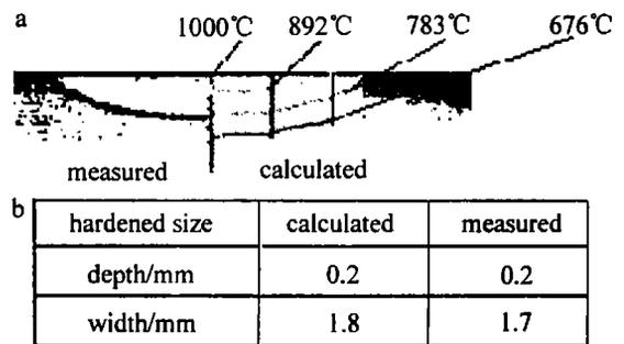
Fig. 6 Laser scanning in  $y = 10\text{mm}$  line compared simulation result with experimental result
