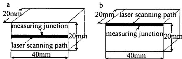
Fig. 2 Sample size and thermal couple welding position
