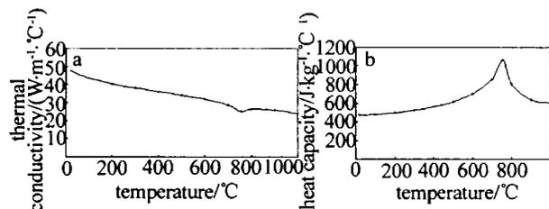
Fig. 3 Thermal properties of steel 45 versus temperature
