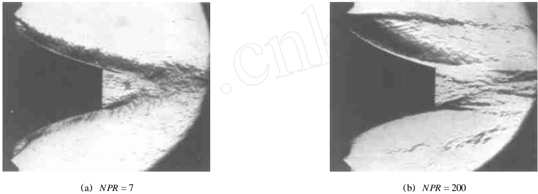
Fig. 4 Schlieren photo of the flow filed of 35% plug
