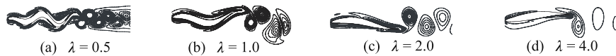
Fig. 12 Vorticity isolines at \lambda = 0.5, 1.0, 2.0, 4.0 (where the vorticity value ranges from -100 to 100 with intervals of 10 dotted and solid lines denote negative and positive contours)
