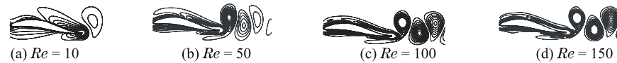
Fig. 13 Vorticity isolines at Re = 10, 50, 100, 150 (where the vorticity value ranges from -50 to 50 with intervals of 5 dotted and solid lines denote negative and positive contours)
