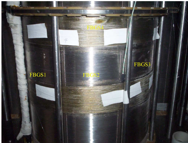
Fig. 3. Picture of FBG sensors attached on the LTS magnet.
