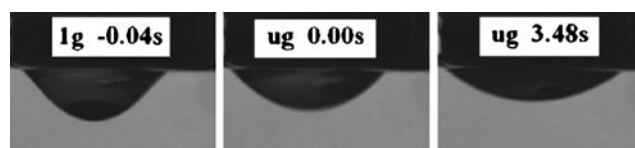
Fig. 7 Ethanol pendant drop on PTFE: variation of the drop contour at different moments during the experiment
