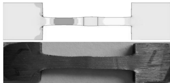
图 9 焊接构件实验与数值模拟的比较 Fig. 9 Experimental and simulated results of welded structure materials
