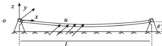
图 1 两端扭转弹性约束的悬跨海管 Fig. 1 An elastically mounted span
