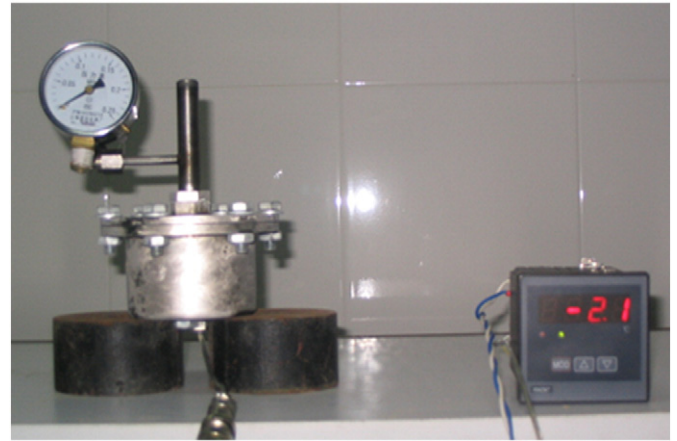
Fig. 1. Layout of model for THF hydrate phase equilibrium test.
