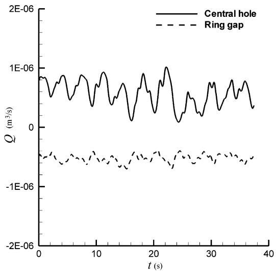
**Fig. 9** Average volumetric flow rate in the central hole and ring gap in the system with inner diameter of 4.44 cm and baffle opening of 10%
