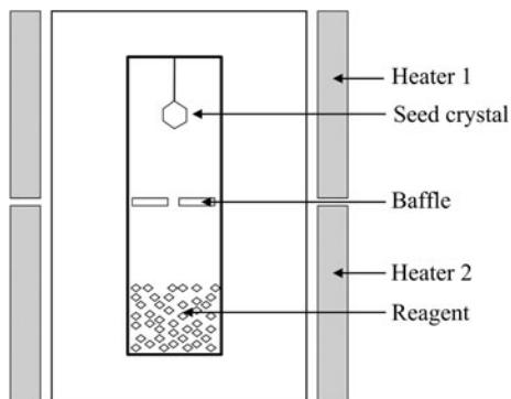
The nutrient particles of GaN in the bottom of the autoclave can be considered as a porous medium. In this case, the Darcy–Brinkman–Forchheimer model can be employed in the porous layer [15]. The dimensionless parameters of the system are listed as follows:
