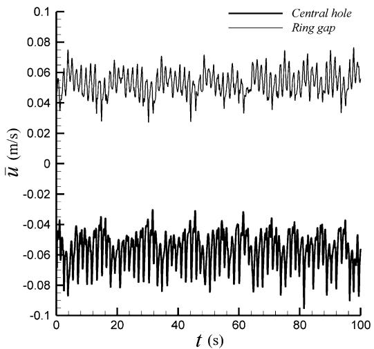
**Fig. 7** Average velocity in the central hole and ring gap in the system with inner diameter of 10 cm and baffle opening of 10%
