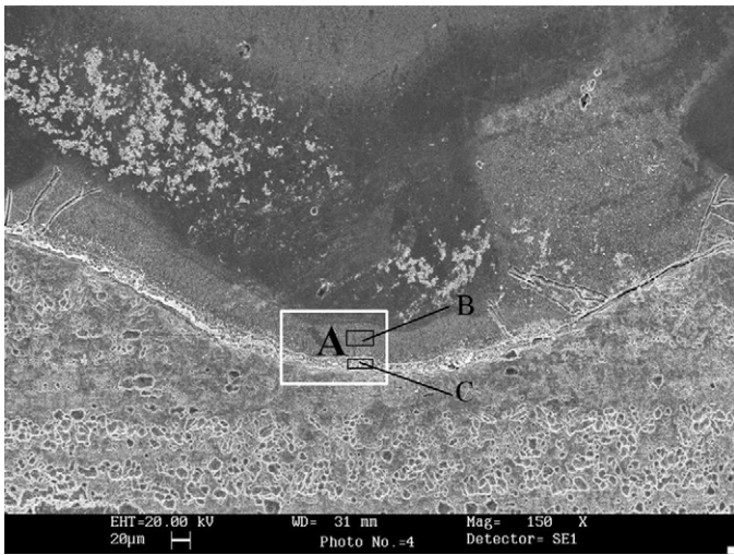
Fig. 9. SEM image of the interface of Ti6Al4V and 42CrMo.
