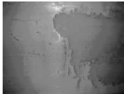
(b) 大面积薄层撕裂( \rho_c = 1.250 \text{ g/cm}^3 )
