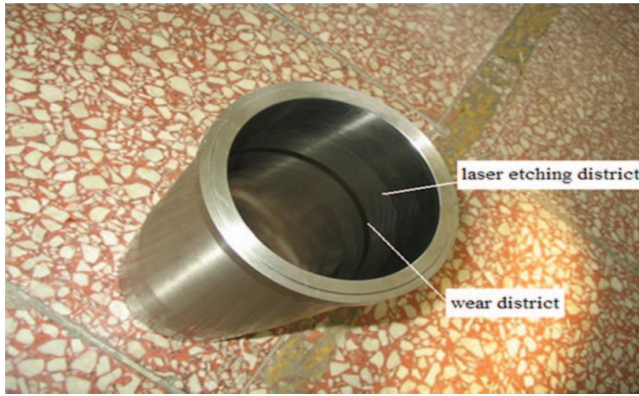
Fig. 4—Image of the laser texturing region and the tested wear region on a cylinder. (color figure available online.)
