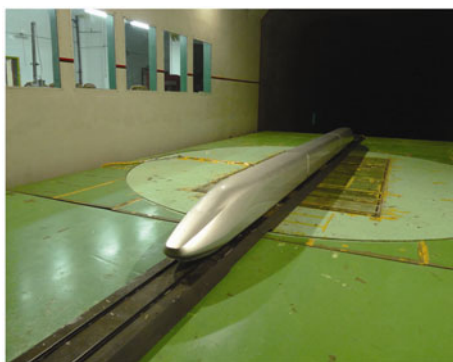
Figure 4 Wind tunnel model.
