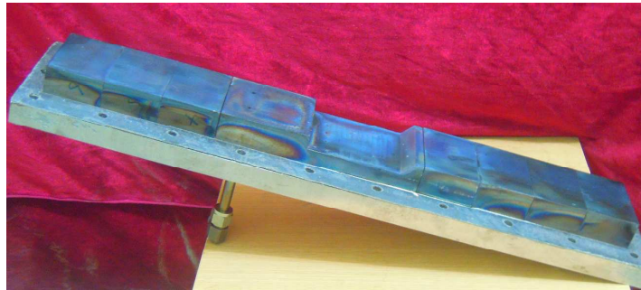
Figure 1. Schematic of the model combustor (top) and picture of a changeable integrated fuel injection/flameholder module (bottom). All length dimensions are in mm.
