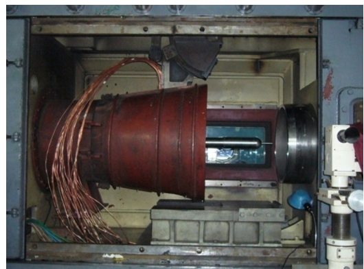
Fig. 2 Test model installed in the hypersonic wind tunnel in CAAA.
