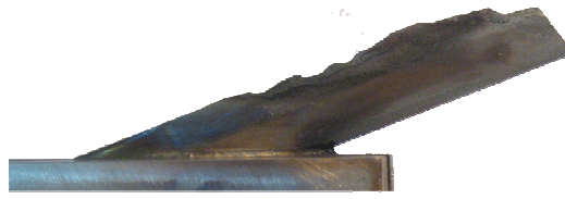
Fig. 11 Photograph of the strut with cooling design of Strut4 after being tested in a supersonic tunnel for 60s
